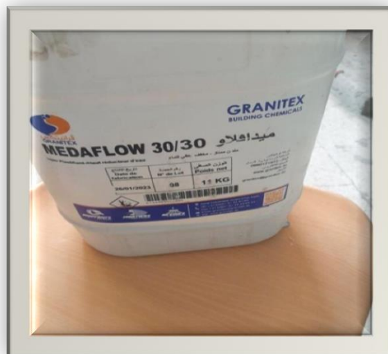
Figure II. 15: L'adjuvant: super plastifiant MEDAFLOW 30/30.
