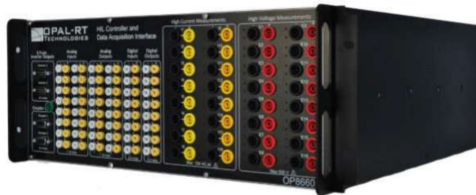
Fig. 4.6: OP8660 HIL controller and data acquisition interface
