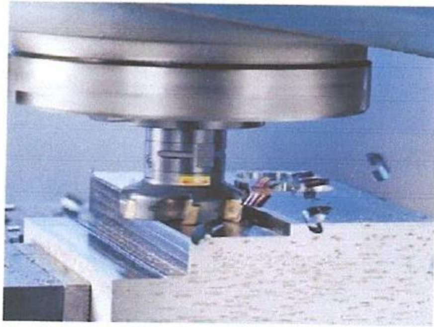
Figure 2.10 formation de copeaux
