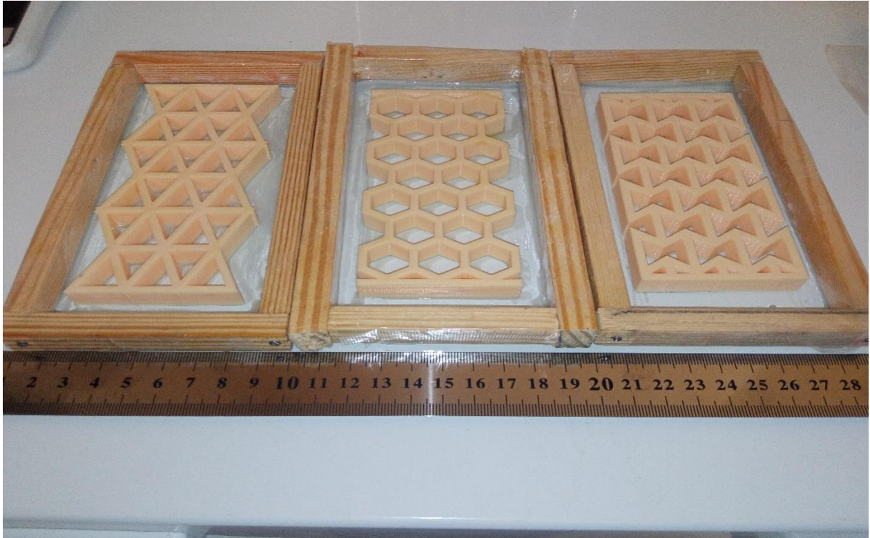
Figure II.4: Position the printed samples securely within a wooden mold
