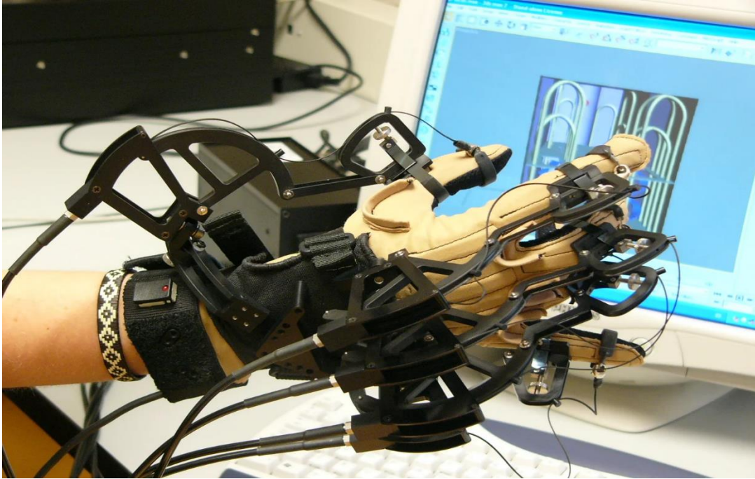
Figure 4 : A CyberGrasp haptic exoskeleton [20] providing force-feedback for virtual hand modeling
