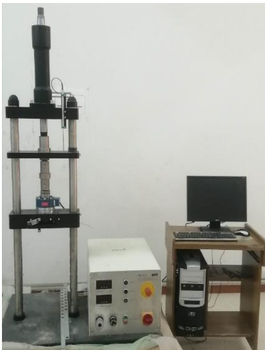
Fig III-9 : Machine essai de compression type de WP 310.
