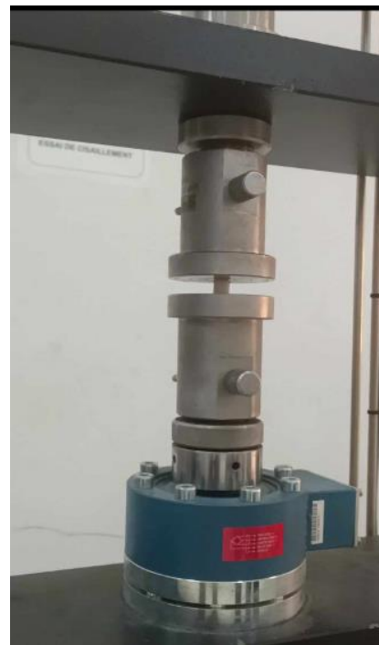
Fig III-9 : Machine essai de compression type de WP 310.
