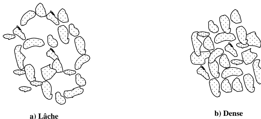
Figure 2.1 Structure de sable
