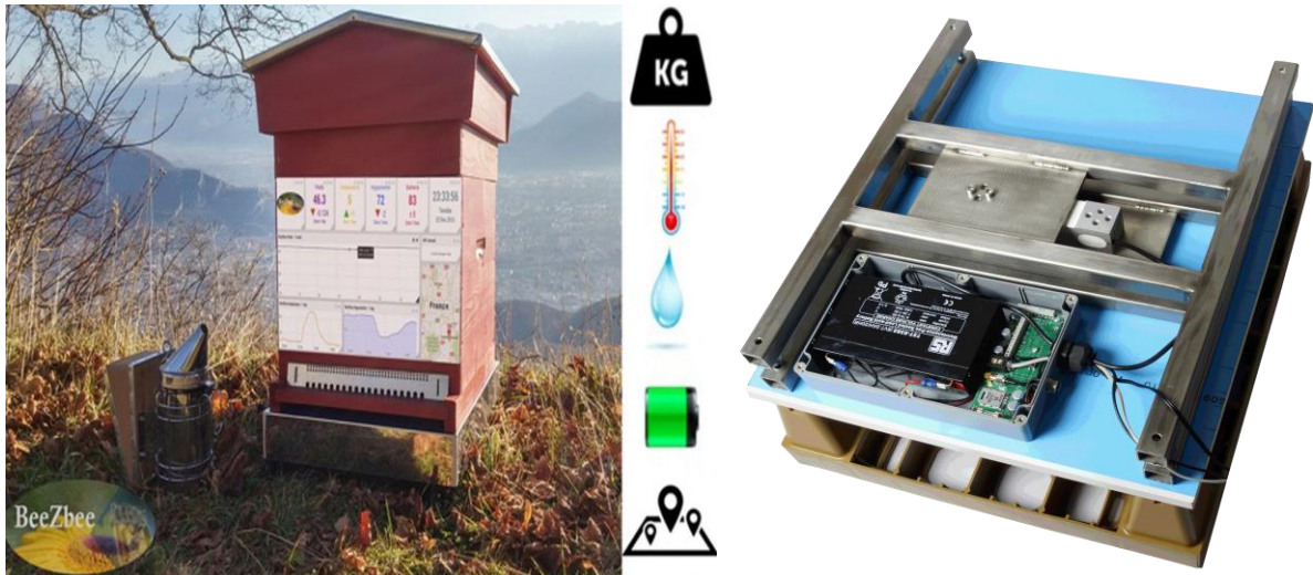
Figure 4. Bee Online connected measuring station for beehives.
