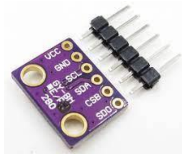
Figure 8 : Pinout of the GY-BMP280 module
