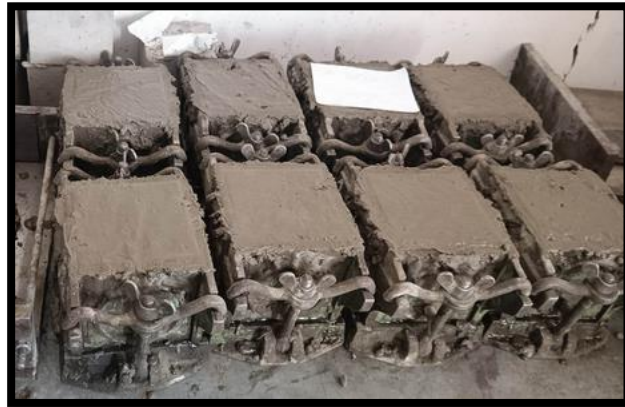
Figure III.9. Confection des bétons.
