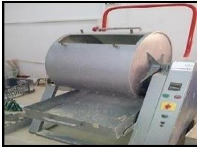
Figure III.6. Appareil Los Angeles.
