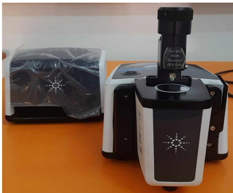
Fig.II.12. Cary630KBr Engine, Agilent Technologies FT-IR spectrometer (Univ-M'sila).
