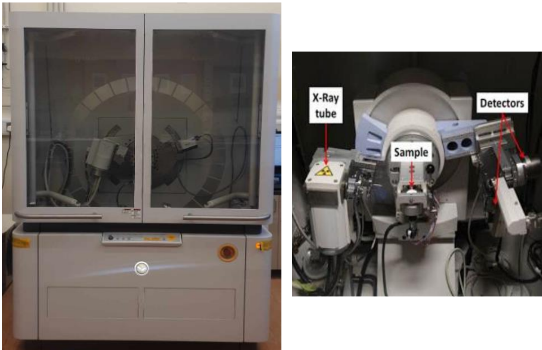
Fig.II.10. Panalytical X'pert Pro, XRD.
