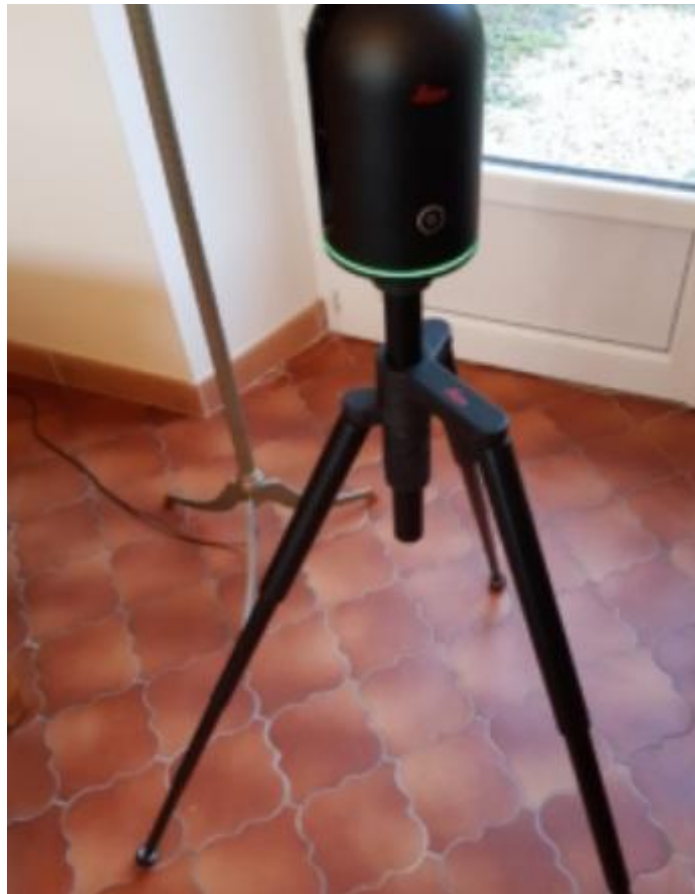
Figure 34: scanner 3D BLK360 sur un support stable (trépied).
