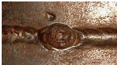
Figure (II.26): Effondrement.
