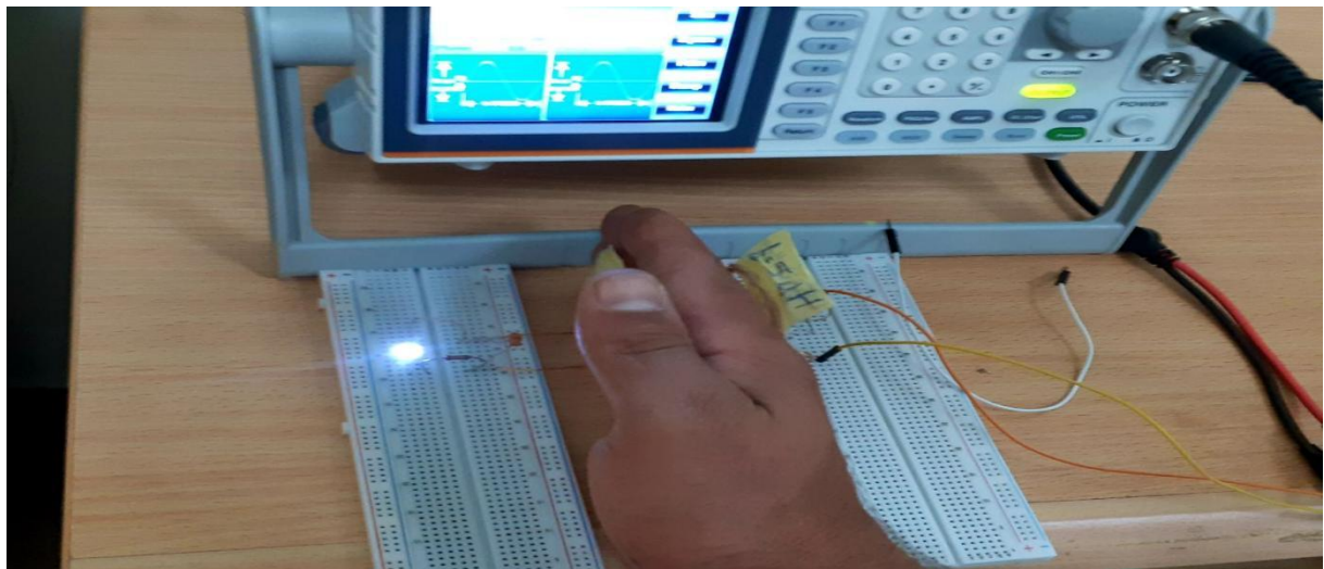
Figure III-9: WPT System Testing with A Human Hand Obstacle
