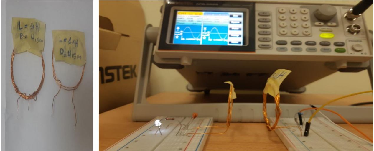
Figure III-8. WPT prototype using solenoid coils
