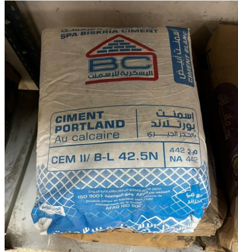
Figure II.7 : Ciment Portland, CEM II / B-L 42.5N
