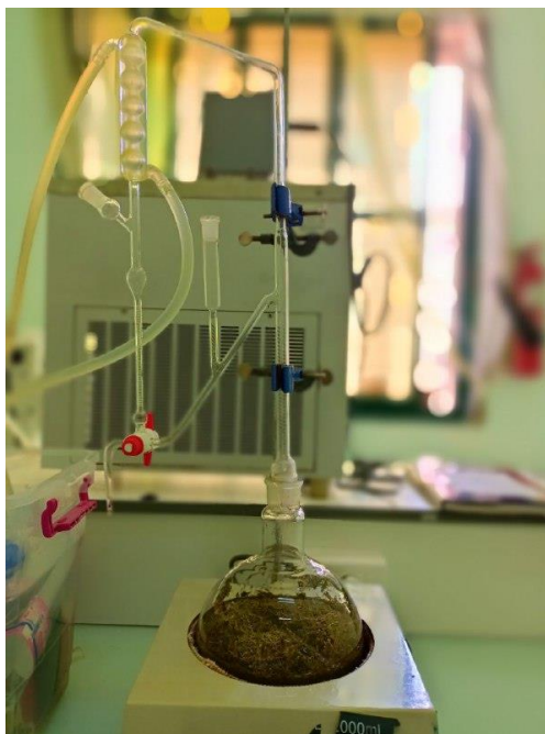
Figure 5: Montage Clevenger (photo originale)
