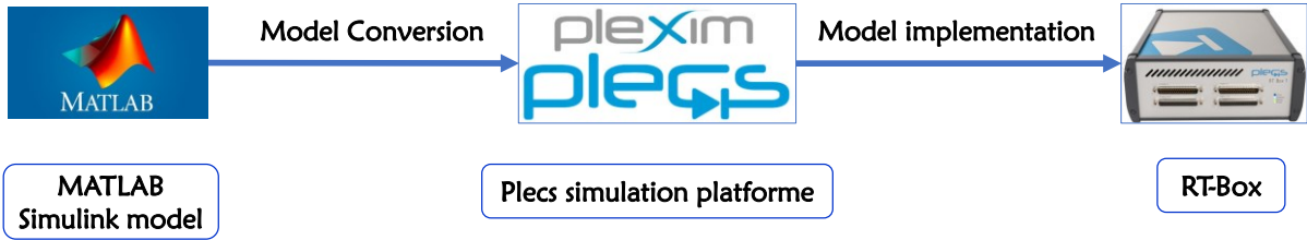
Figure IV.3. HIL implementation in RT-BOX1.
