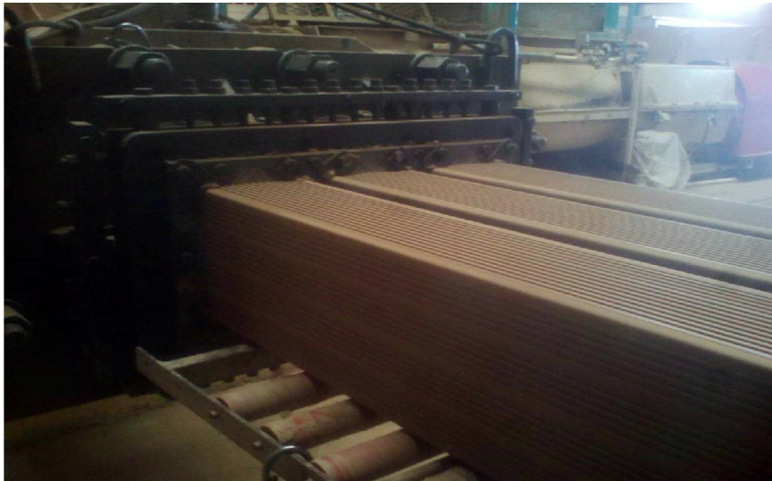
Figure I.7: represents the brick during the cutting processes
