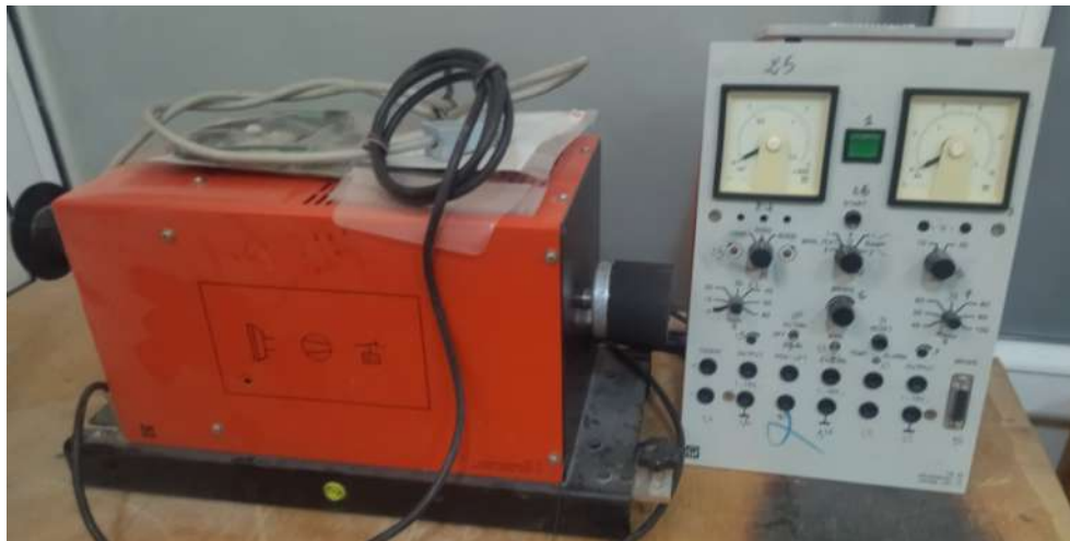
Fig B.9. Powder Brake and its Torque Control Unit
