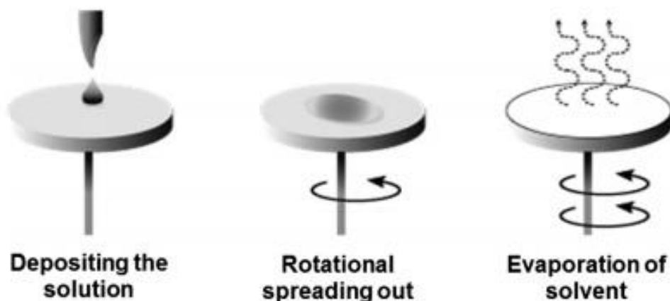
Figure III. 4. Scheme of the Spin-coating process [120].
