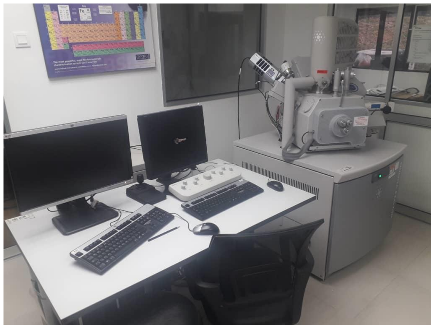
Figure III. 14. Image of the used scanning electron microscopy Zeiss Supra 35 VP.
