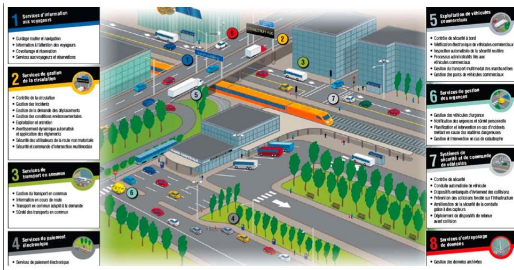
Figure 2.4 Architecture générale d'un ITS
