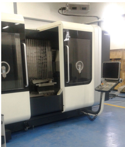
Fig. 25 The Five-axis vertical machining center (VMC) type DMG
