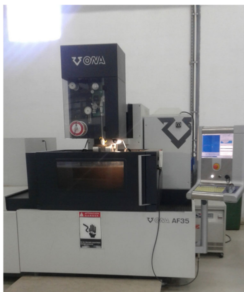
Fig. 26 The ONA AF35 wire electrical discharge machining machine
