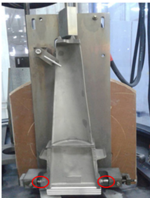
Fig. 5 Machining device for drilling cooling holes at the airfoil of the blade by ECD
