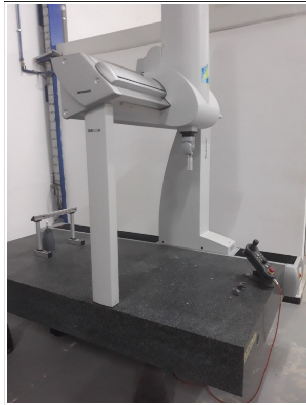
Figure 3.9: Coordinate Measuring Machine (CMM) for 3D Scanning in the Scanning Phase.
