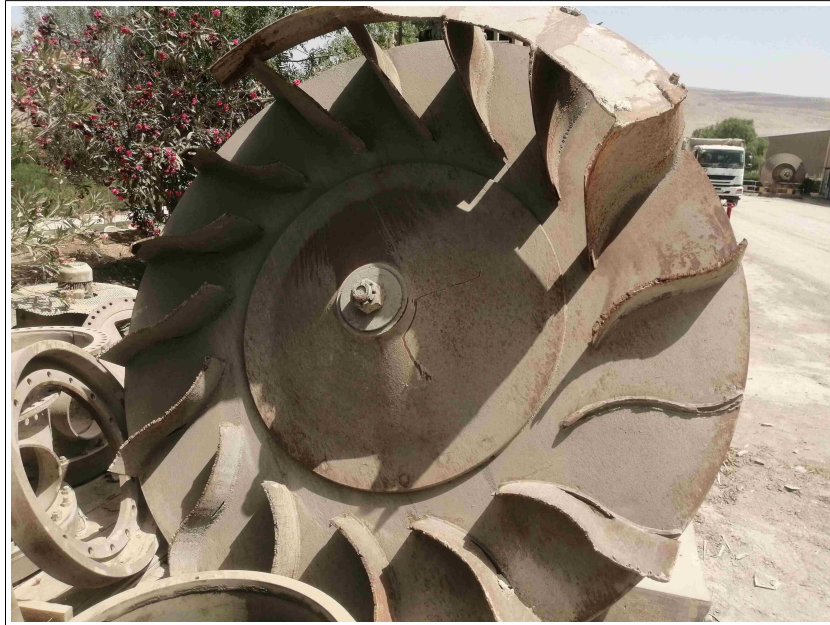
Figure 1.2: Fan Impeller failure
