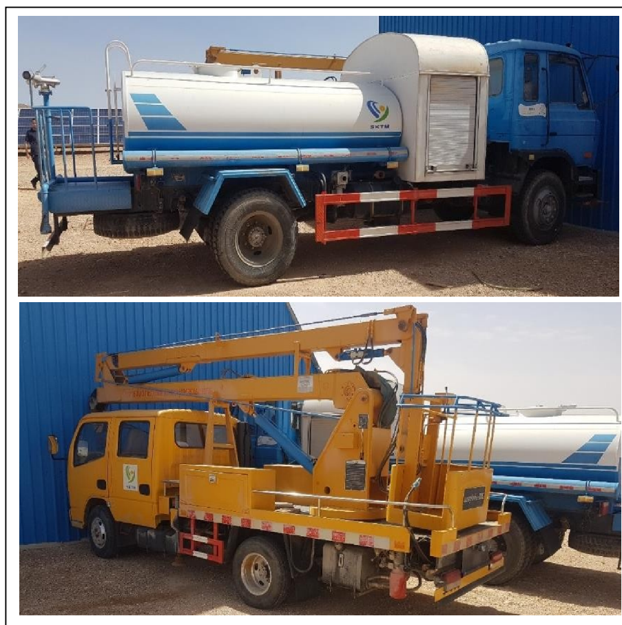
Figure II.17. Equipment for maintaining and cleaning panels and the photovoltaic power plant.
