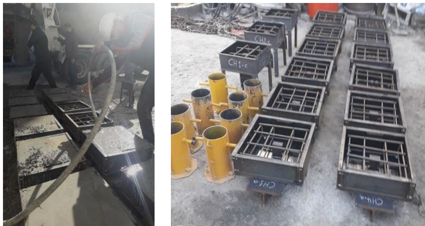
Figure 2.1: Casting in a horizontal position (before and during casting).
