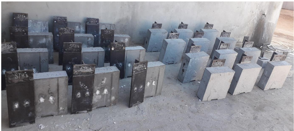
Picture C6: Push and pull - out specimens after tests.
