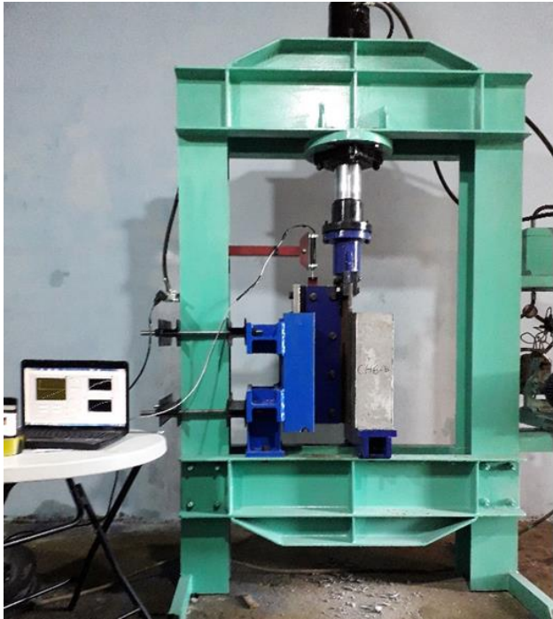
Figure 3.5: Applying load on the push-out specimen.
