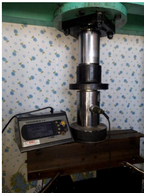
Figure 2.11: Calibration of the load sensor.
