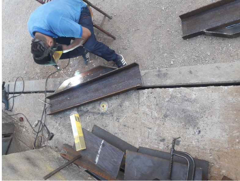
Picture C1: Welding of the hydraulic press beam.
