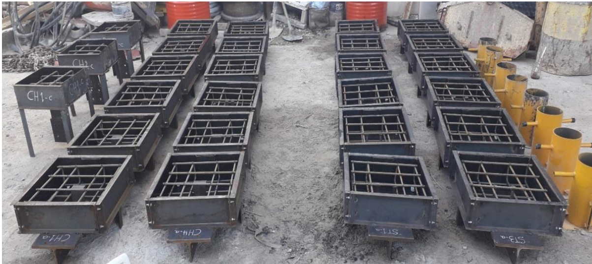
Picture C5: Push and pull - out specimens before casting.
