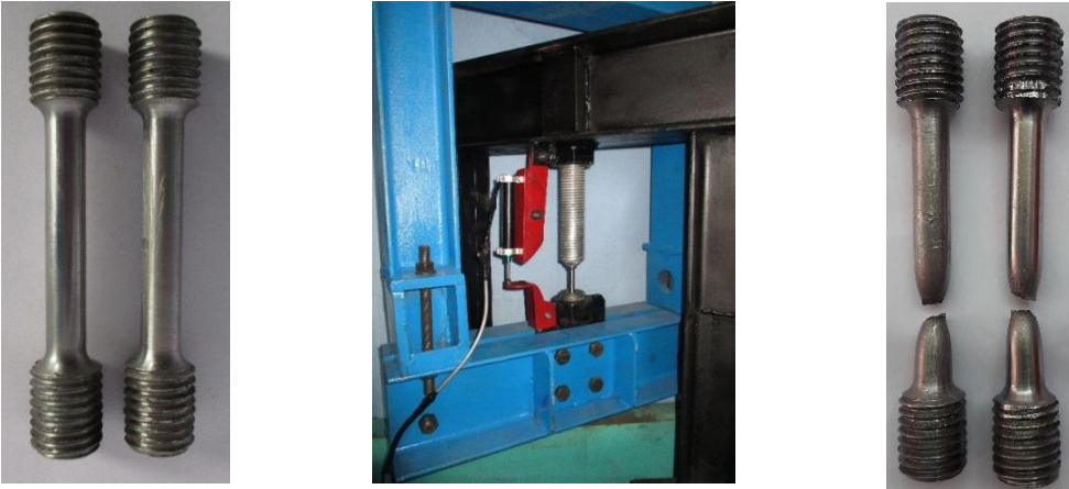
Figure 2.3: Tensile strength testing of headed studs.
