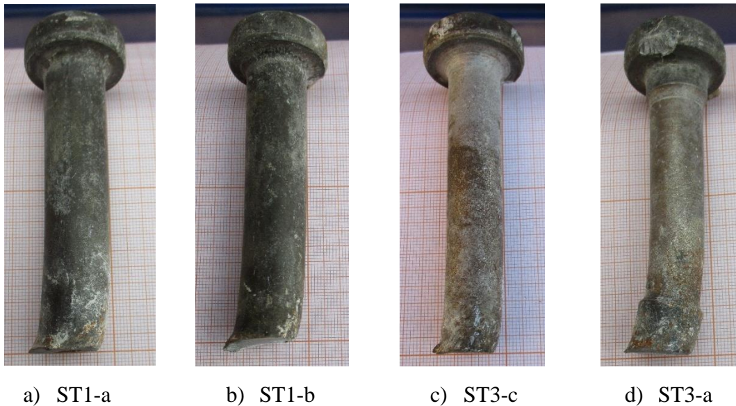
Figure 4.7: Headed studs' deformation.
