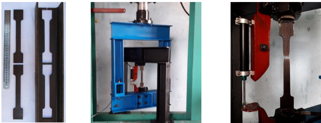
Figure 2.2: Tensile strength testing of channel shear connectors.
