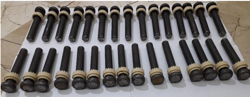
Figure 2.6: The headed stud shear connectors used in the specimens.
