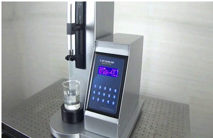
Figure I.14 : Image de la technique du Dip Coating [23].
