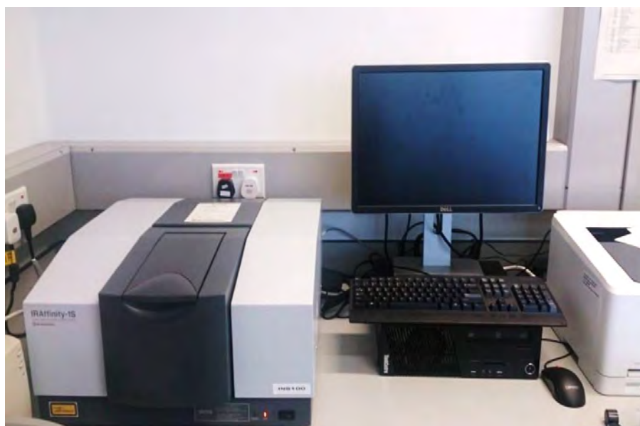
Fig. II.12: SHIMADZU IRAffinity-1S FT-IR spectrometer.
