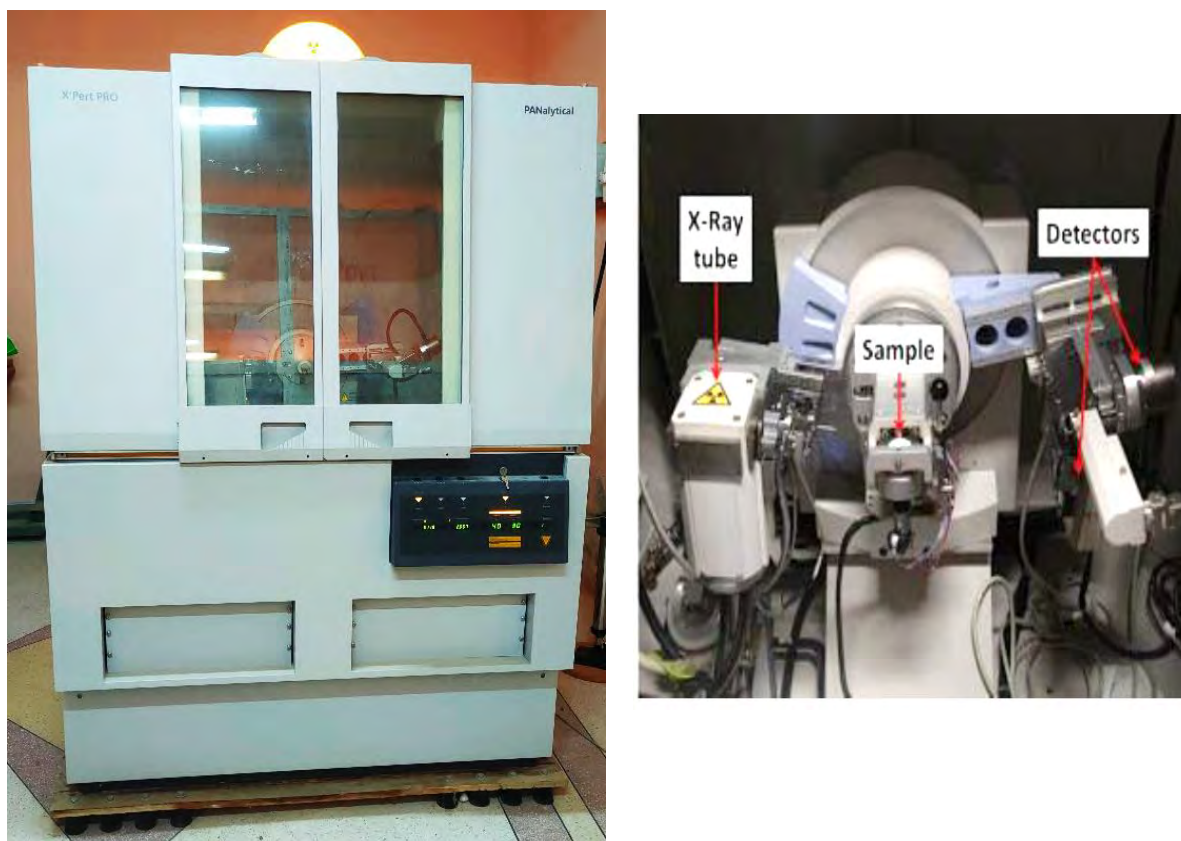
Fig. II.10: Panalytical X'pert Pro, X-ray Diffractometer.
