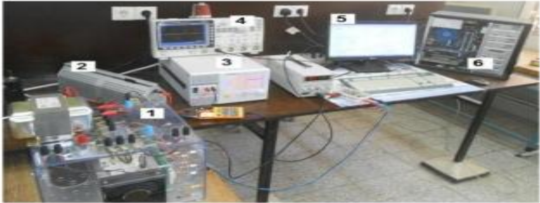
Figure III.1. Photograph of the emulator used for data collection: 1) buck converters, 2) load 3) programmable power source, 4) scope, 5) ControlDesk, 6) DS1104 platform .[98]
