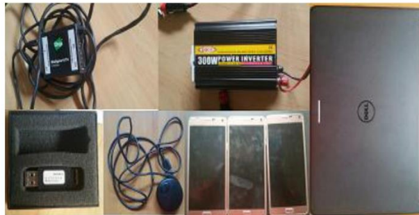
Figure III.8: Drive Test materials [30]
