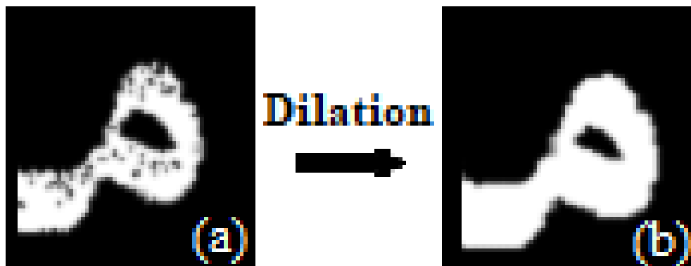
Figure 4-10: Character Enhancement (Dilation).
