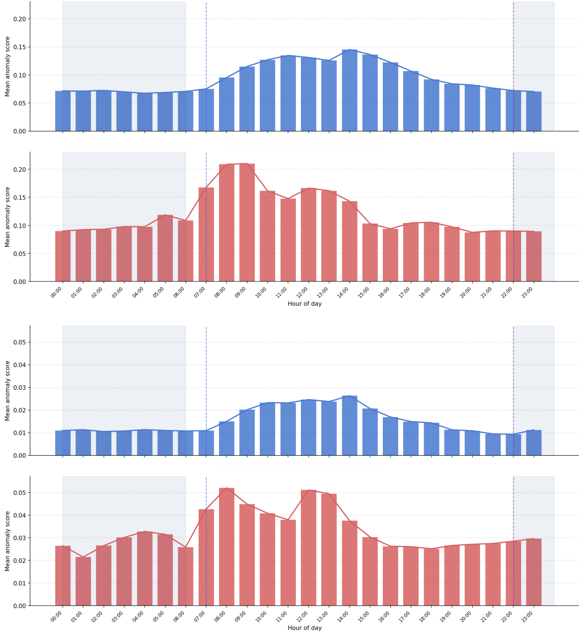
Figure 4.3: Temporal distribution of mean anomaly scores across the 24-hour daily cycle for GDN (top) and MTAD-GAT (bottom). Blue curves correspond to normal behavior (Actor 1), while red curves represent anomalous behavior (Actor 2).
