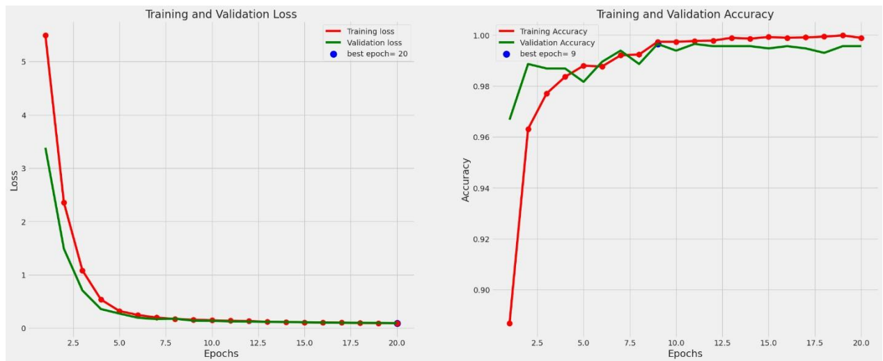
FIG 3.7 – Balanced EfficientNet B3 - Training and Validation Loss and Accuracy (Epochs=20, Batch Size=16).
