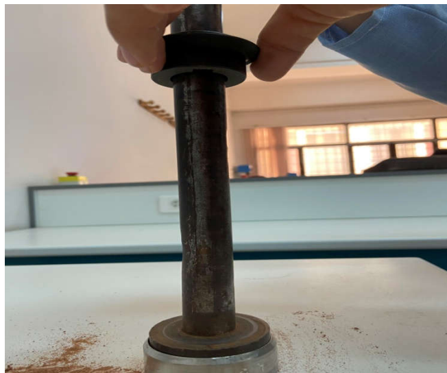
Fig. III. 5 dame de compactage.
