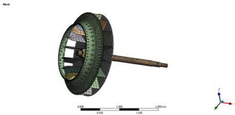
Figure III.13: Maillage du rotor
