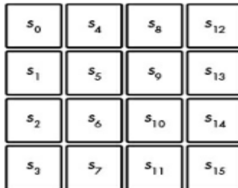
Figure 1.9: The internal state of AES viewed as a 4 \times 4 array of 16 bytes.
