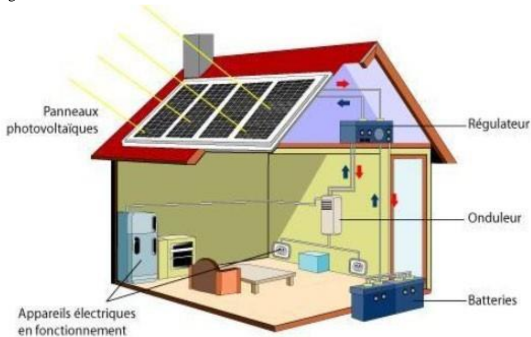
Figure II.1 : structure de l'installation photovoltaïque autonome.
