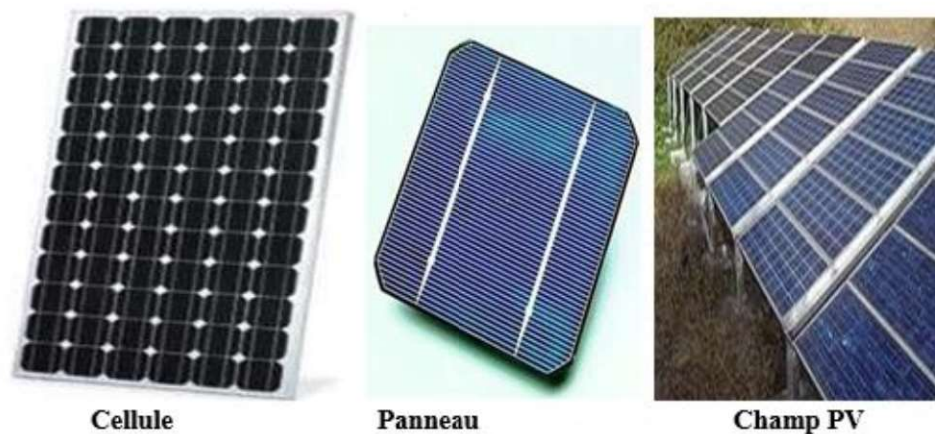
Figure 1.7: Photovoltaic cell, module and field
