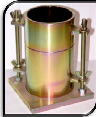
Figure II.10: Moule Proctor normal .
