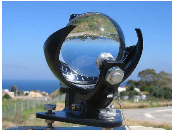
Figure I.13 : Héliographe de Campbell-Stokes. [22]
