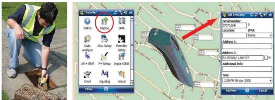
Figure.2.23 Deployment with lift and shift method and mapping with GPS. [14]
