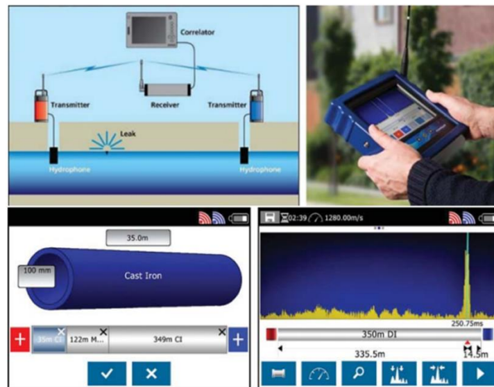
Figure.2.18 Reading from radio-based correlator on ductile iron pipe with 350m long. [14]
