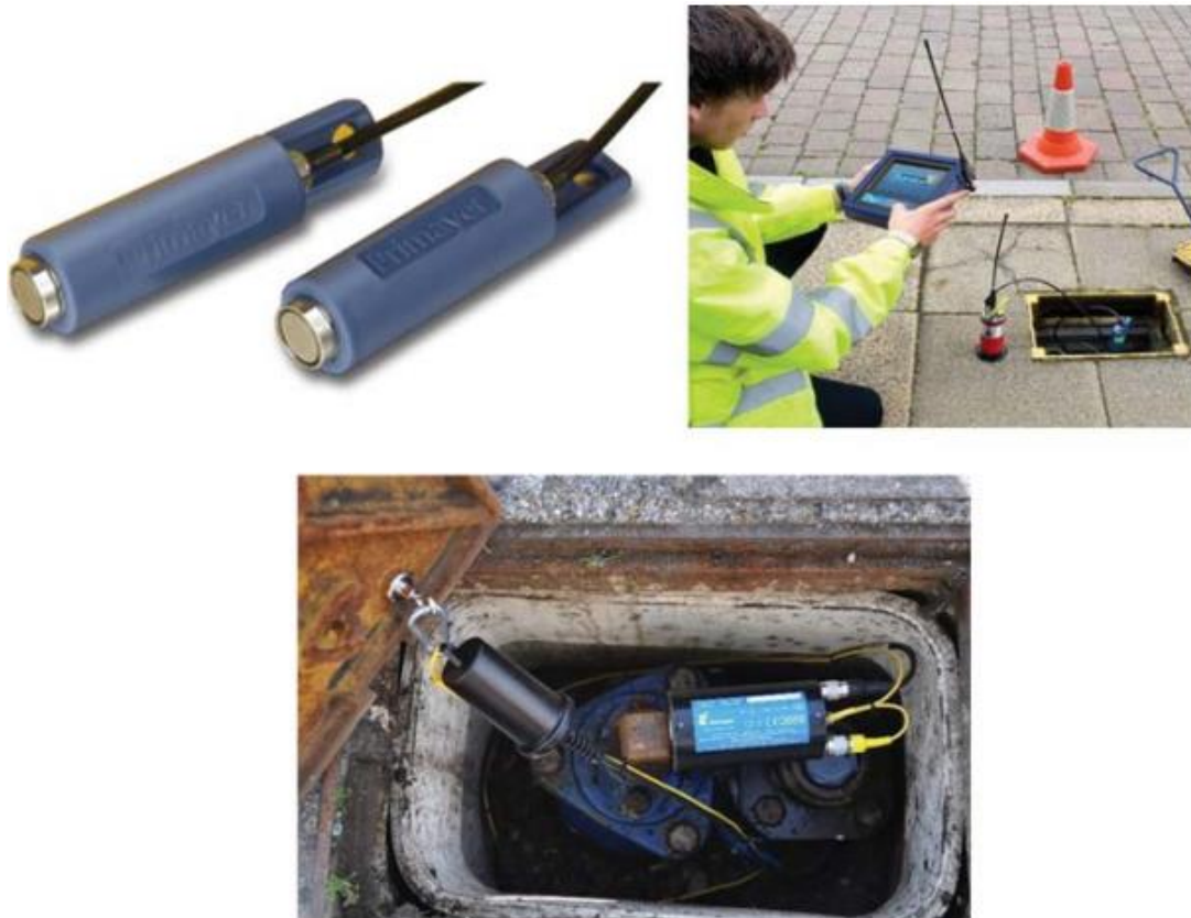
Figure.2.15 Accelerometer sensors paired with a radio-based correlator. [14]
