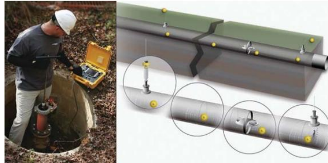
Figure.2.20 Deployment of a free-swimming sensor in the pipe. [14]
