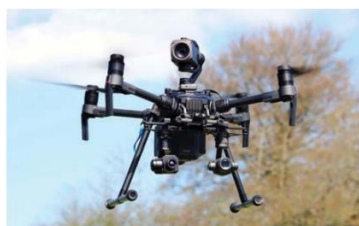
Figure.2.25 Leak detection with drones equipped with cameras. [14]
