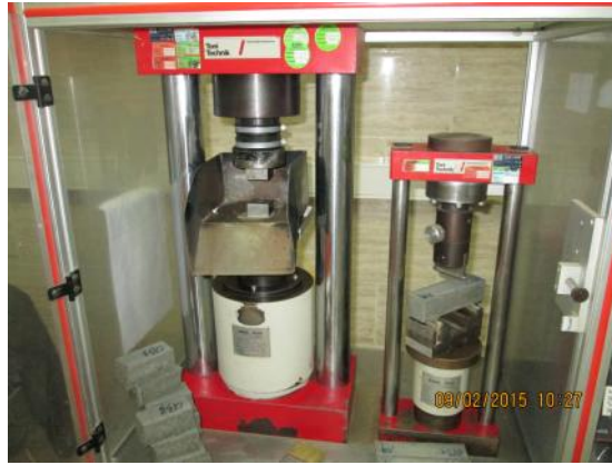
Figure III.6 : Appareil de flexion et de compression (Toni Technic).
