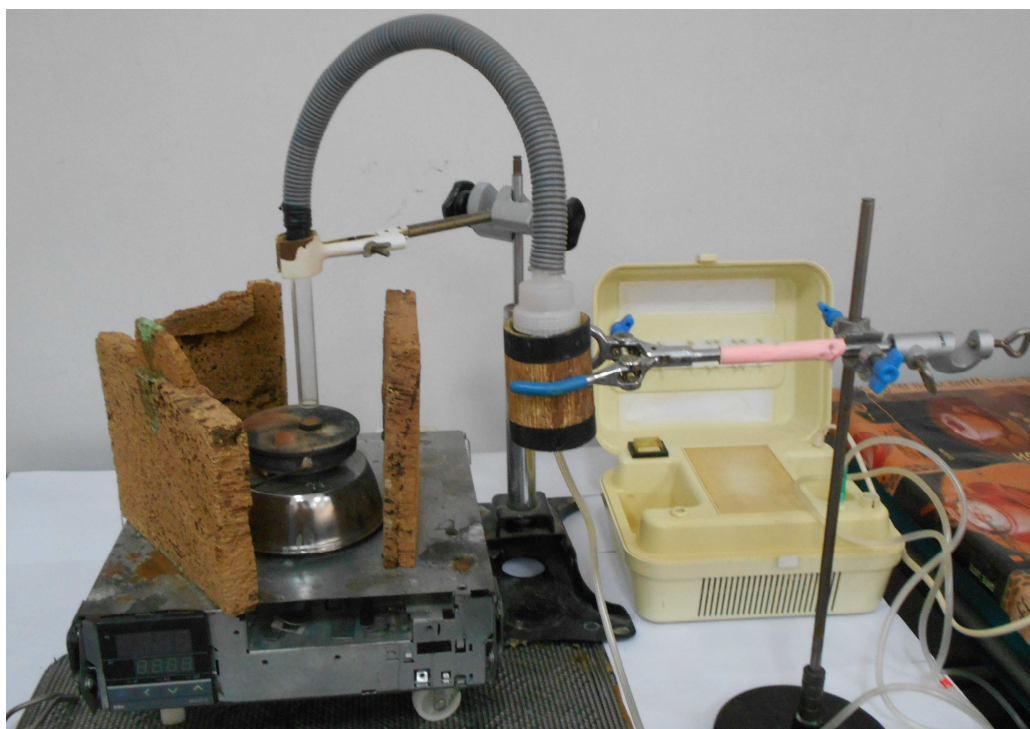
Fig. 9 The spray technique used to deposit the coating
