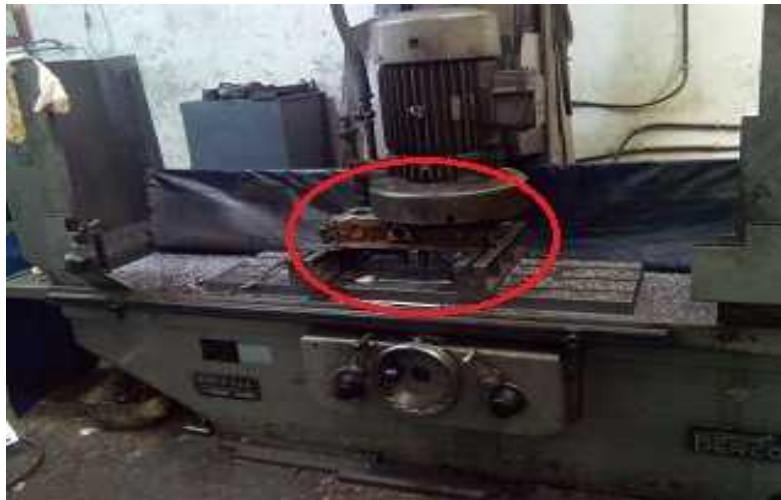
Figure III.6. Rabotage de culasse.
