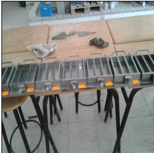
Figure III.6. Moules prismatique (4x4x16).
