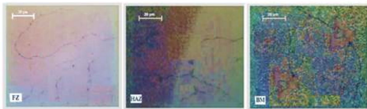
Fig. 10. The microstructures in the (BM, HAZ, FZ) of INC738LC Ni superalloy after post-welding heat treatment
