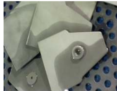
Fig. 1. The plates cut from the blade root of the Ni superalloy INC738LC with 2 mm thick
