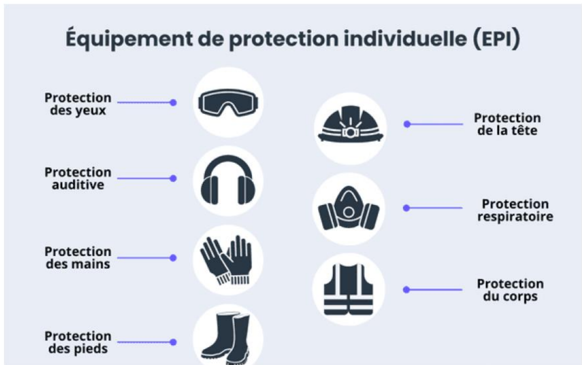
Figure.III.24: Personal Protective Equipment (PPE)
