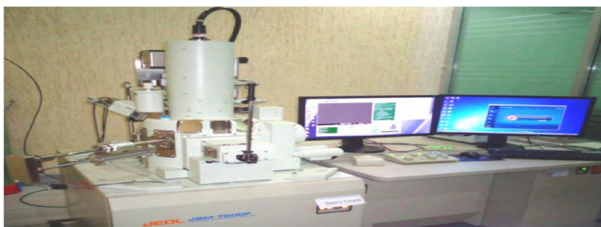
Figure III.3: Setup of a field emission scanning electron microscope.
