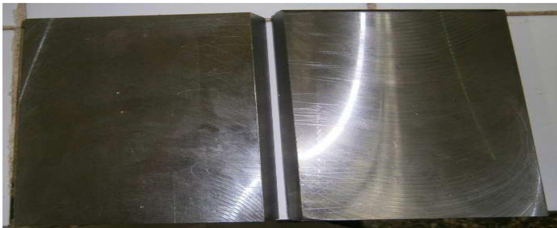
Fig.IV.7 Deux plaquette acier inoxydable310S.
