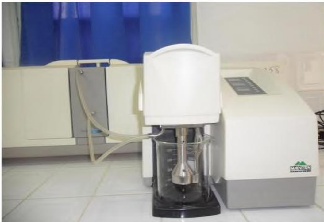
Figure II.7: Granulométrie laser Malvern Mastersizer 2000/3000.
