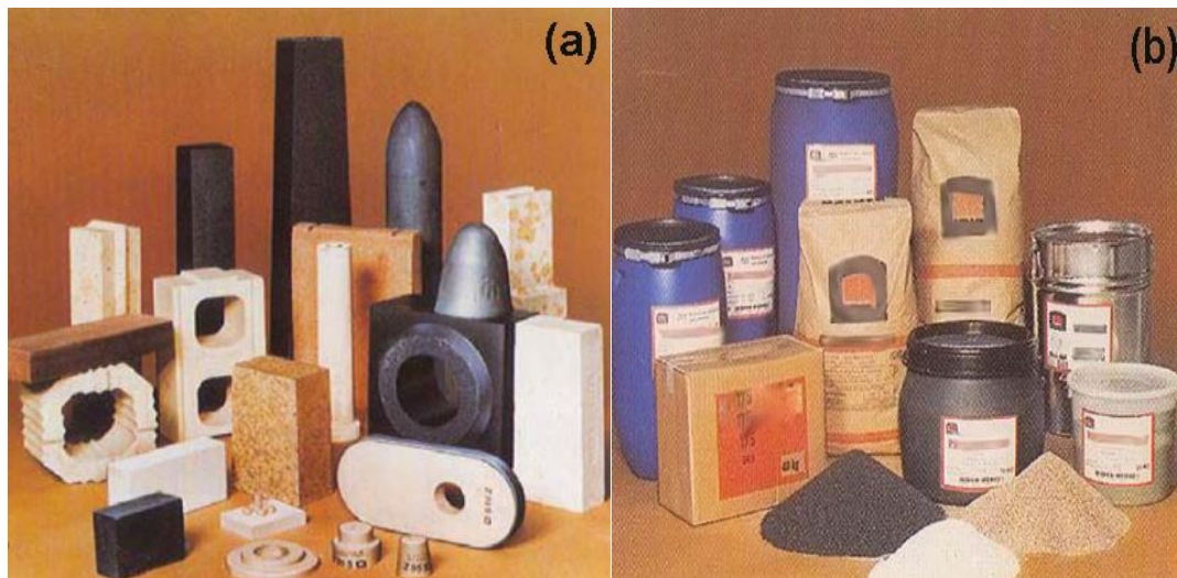
Figure I.4 (a) shaped and (b) unshaped refractory materials [19].
