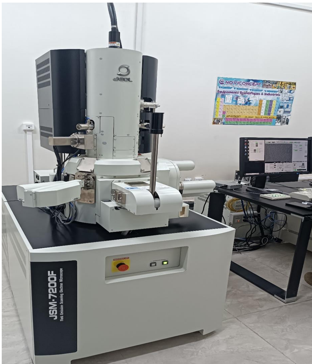
Figure II.14 Scanning electron microscopy (SEM) combined with Energy Dispersive Spectroscopy (EDS) (univ of Bejaia).
