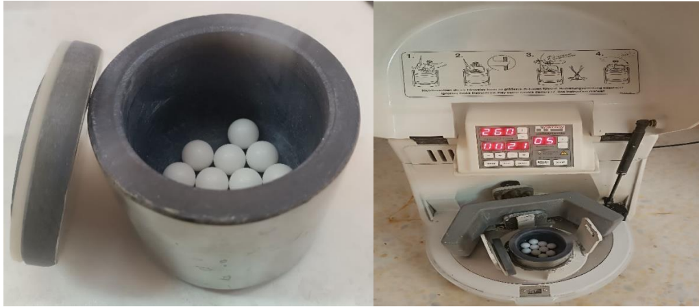
Figure II.2 Planetary ball mill (Fritch P6) and grinding bowl with zirconia balls.
