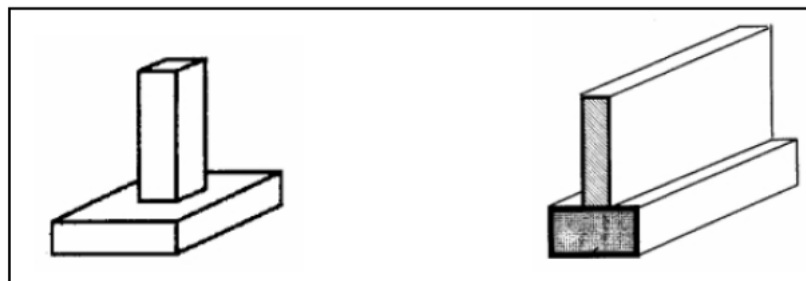
Figure 5. Isolated footing, and continuous footing under wall.
